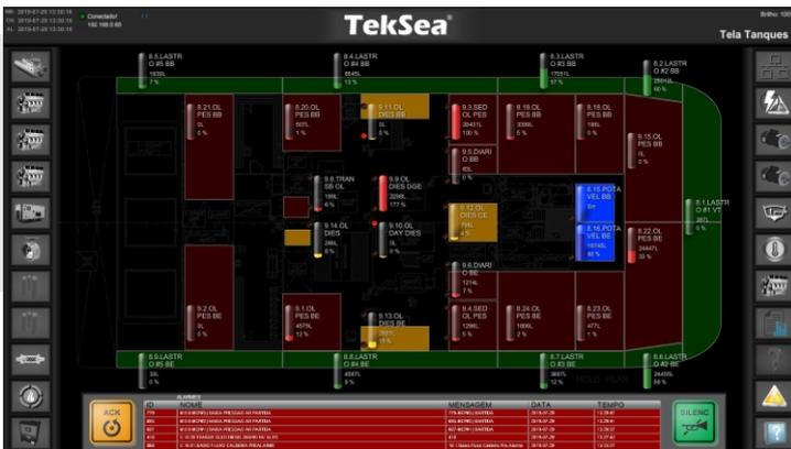
✓ Tanques de lastro e combustivel
